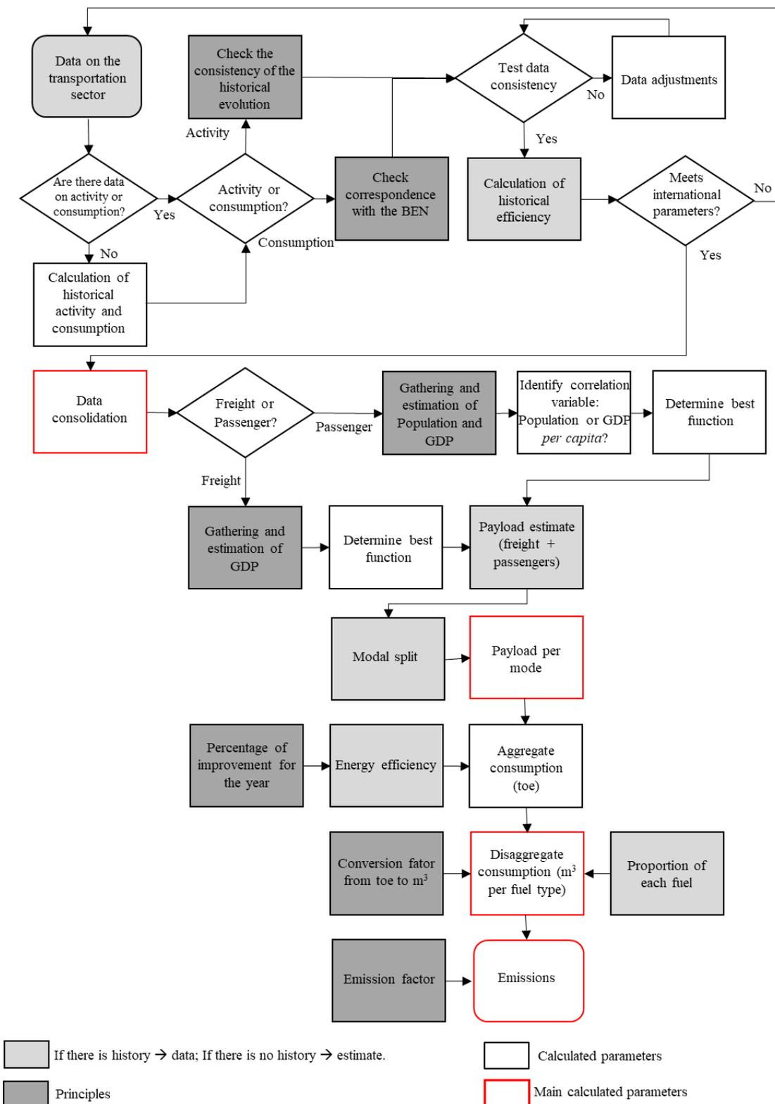
**Figure 3.** Procedure adopted to estimate energy consumption using the *top-down methodology*.
