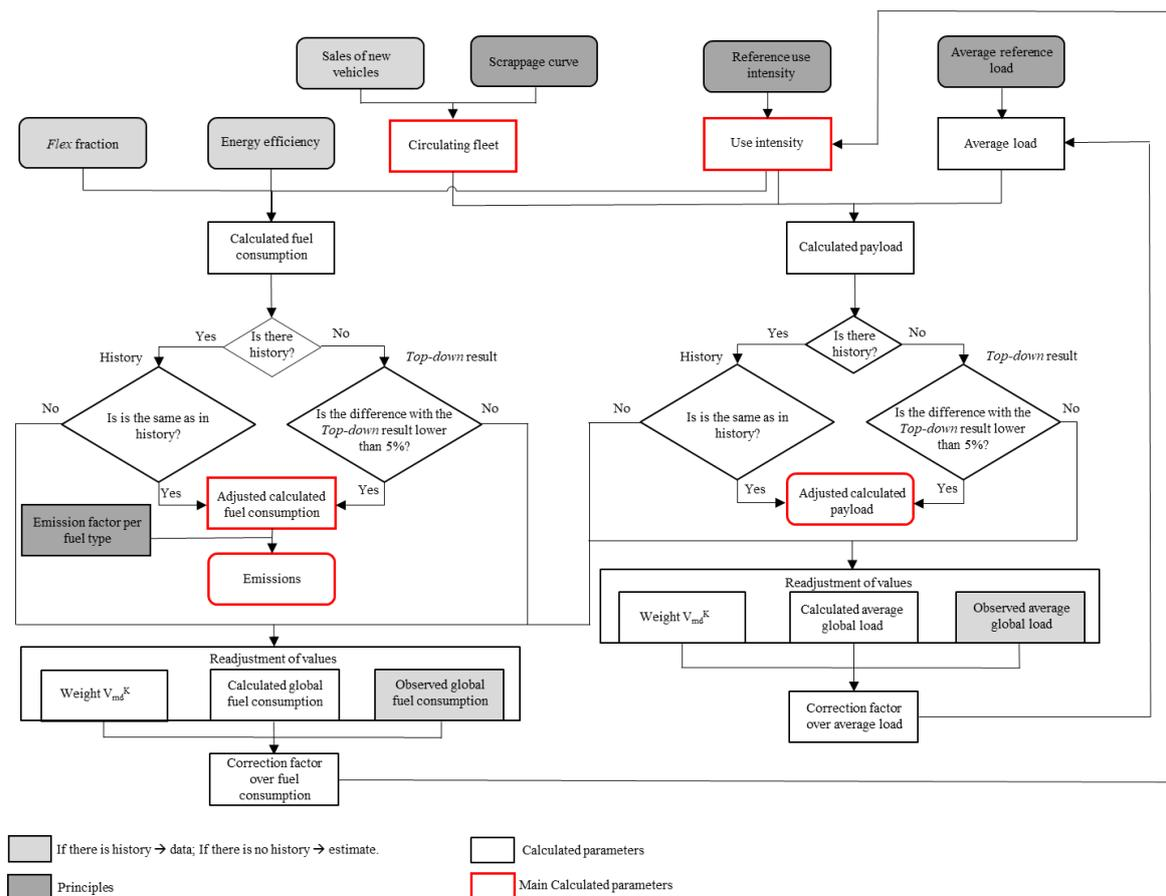
**Figure 4.** Procedure adopted to estimate energy consumption using the *bottom-up* methodology.
