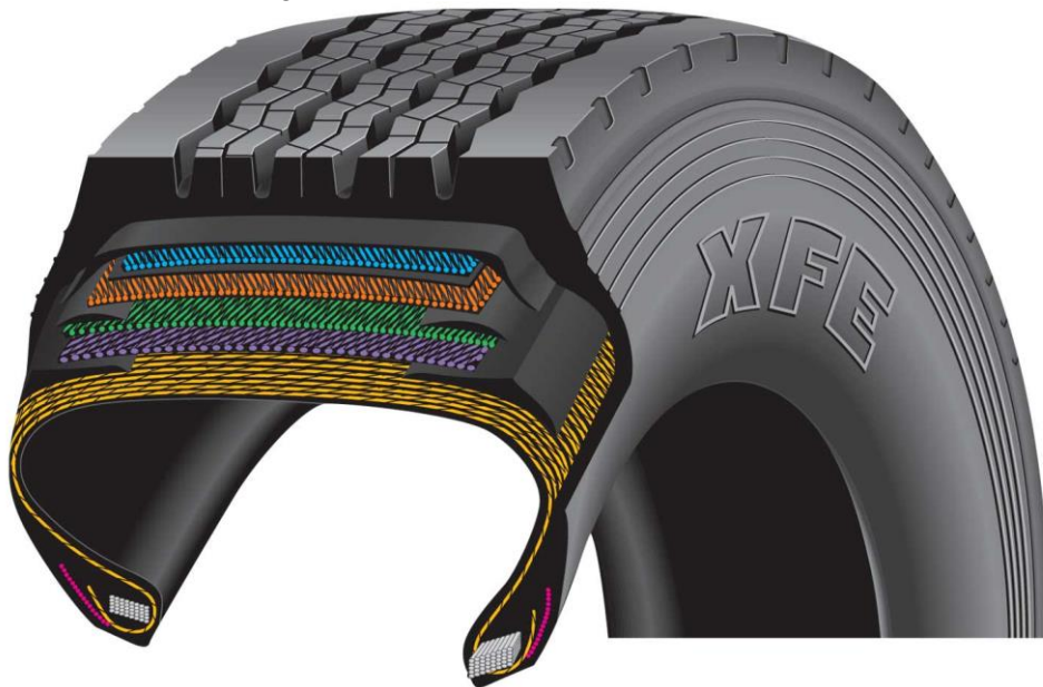
Figure 2 – Truck tire's overall structure [2]
