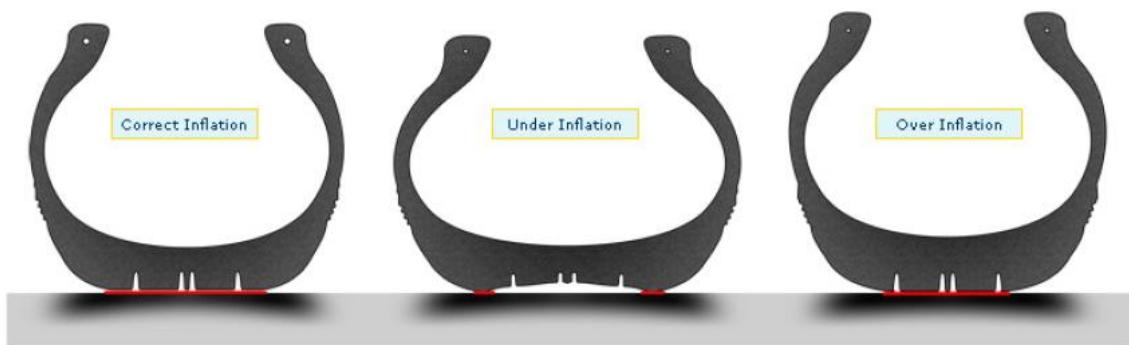
Figure 4 – Tire's geometry due to inflation pressure [5]
