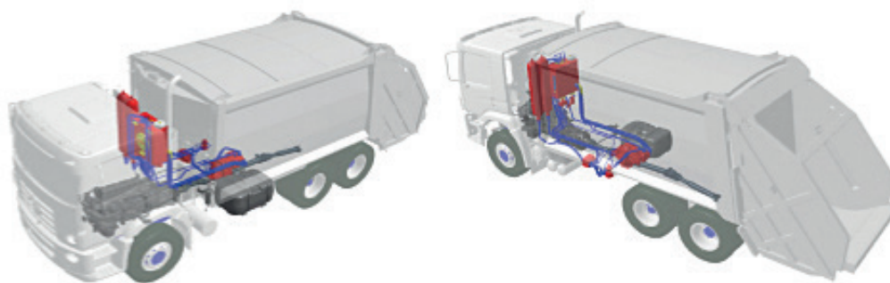
Figure 3: Illustration of the diesel-hydraulic hybrid propulsion system
